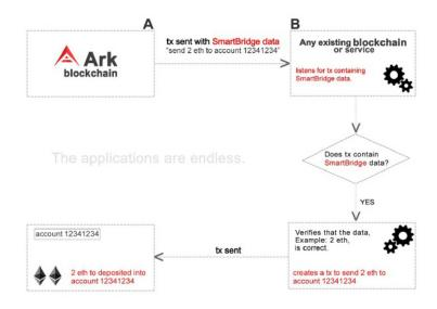
This is a very simplistic example, but SmartBridge data can be more complex (send equivalent amount, split it over several accounts, create an ETH smart contract as addressed by SmartBridge), etc...
